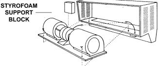
Figure 4 - Removing Motor/Blower Assembly
